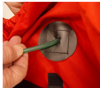
13. Install green tubing through patch on door
