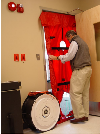
19. Install door frame with panel into the test door
