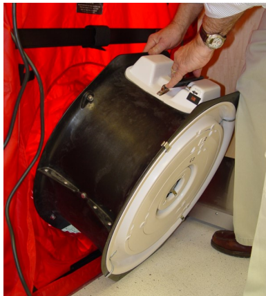
22. Install fan into frame with white flow rings facing you
