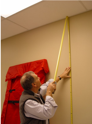
14. Measure the zone, here the maximum protected height
