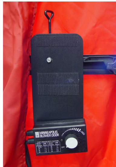
23. Clamp speed control board to cross bar
