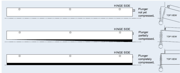
Functioning of an automatic door bottom
