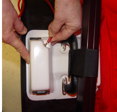
26. Attach other end of the red fan pressure to nipple on fan
