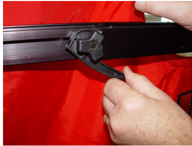
20. Using toggle cams lock frame into the test door
