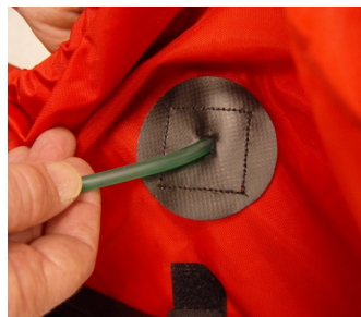
13. Install green tubing through patch on door
