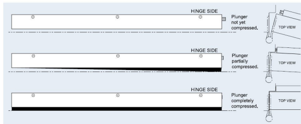
Functioning of an automatic door bottom
